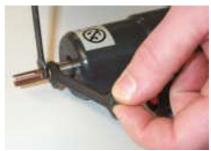
Make sure that pinholder is tight to the gun, use spanners as the figure shows. Otherwise a spark can destroy the axle. Use one spanner 8mm and one 10mm for 8-9,5 mm and M8 pinholders. Two pcs of spanner 10mm for M10 and M12 pinholders.
